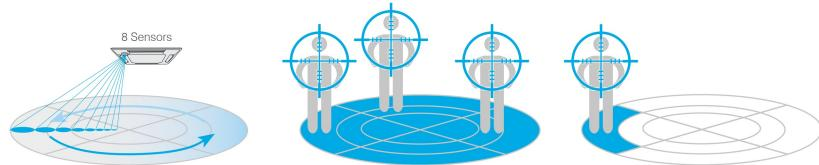
With a total of eight sensors, which rotate a full 360° in three-minute intervals, the 3D i-See Sensor is able to detect people's positions within the room to provide direct or indirect airflow, as preferred.
